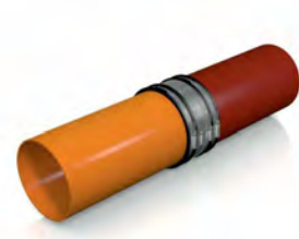
Center coupling over joint. Tighten clamps and shear band reciprocally.
