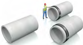
Position plain ended pipes.
