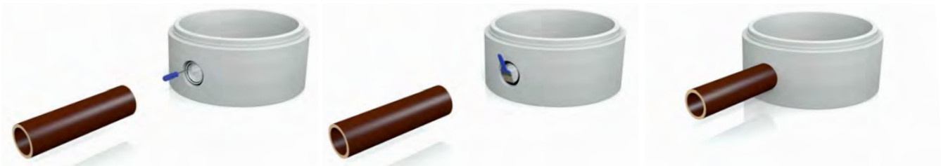
Remove polystyrene from socket.
